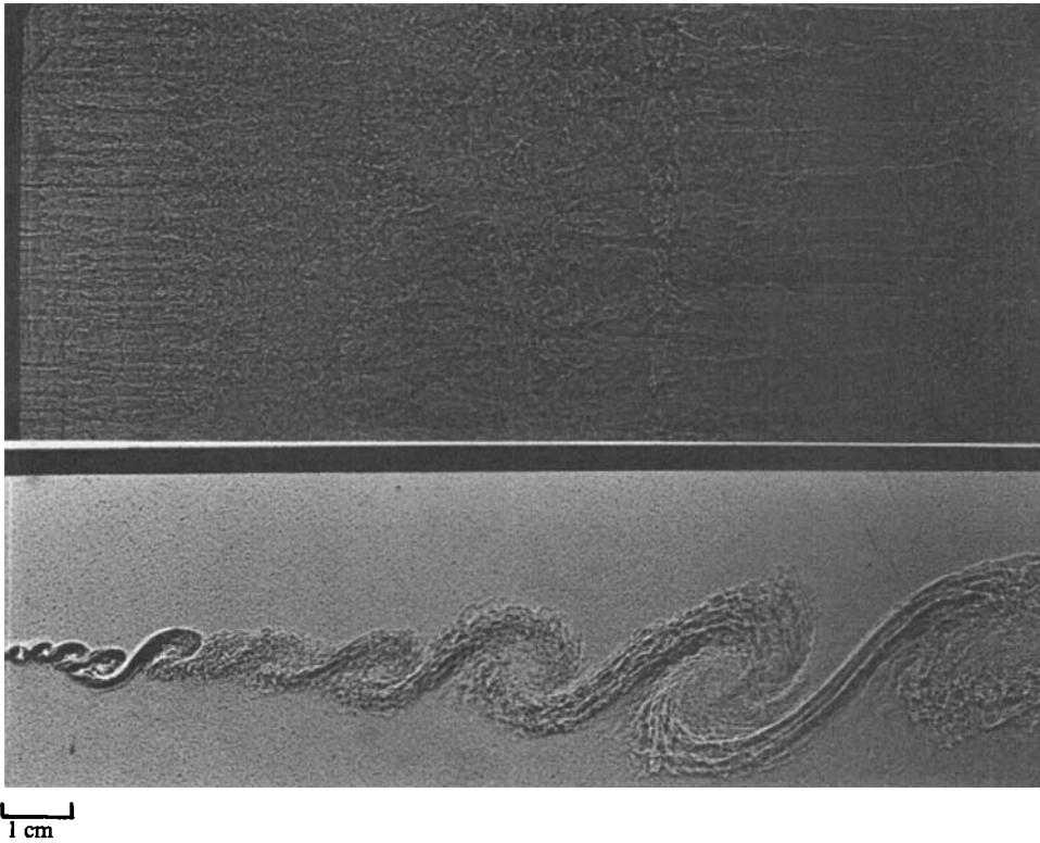
FIGURE 9. Spark shadowgraph picture of the uniform-density mixing layer. U_1 = 1000 cm/s, r = 0.38 , P_0 = 4 atm. Scale as indicated. From Konrad (1976).
