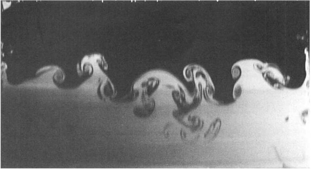
FIGURE 12. Laser-induced fluorescence ( y, z ) cross-section through the braid. U_1 = 29 cm/s, U_2 = 10 cm/s. The entire channel span (11 cm) is shown.
