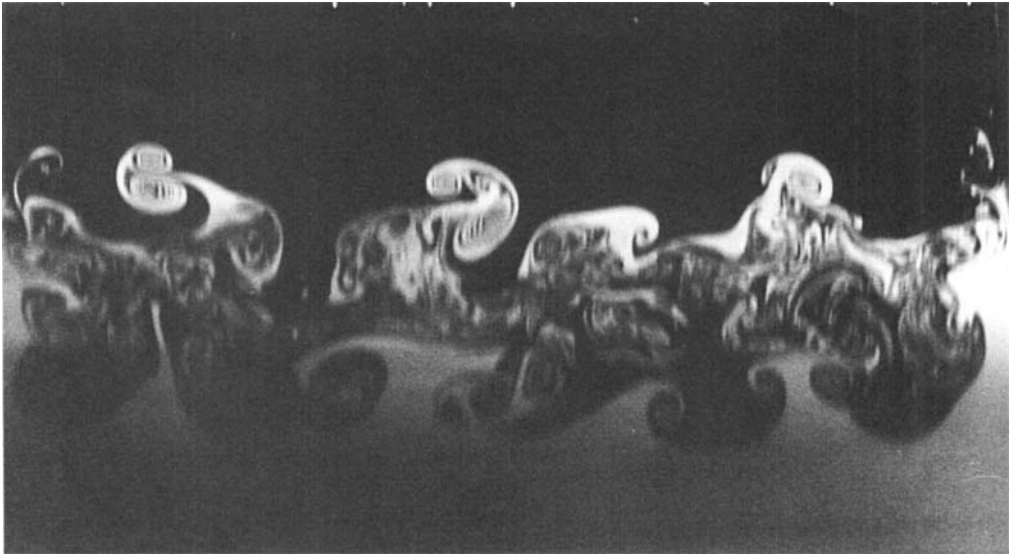
FIGURE 13. Laser-induced fluorescence ( y, z ) cross-section through the core. U_1 = 20 cm/s, U_2 = 8 cm/s. The entire channel span (11 cm) is shown.
